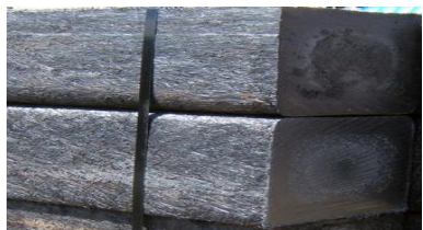
Fig. 14: Wood core sleeper
