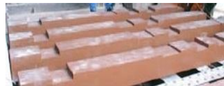
Fig. 5: Polyurethane (FFU) composite sleeper
