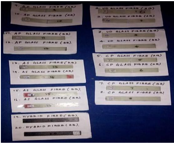
Fig. 1: Fabricated specimens for flexure test and IRT inspection
