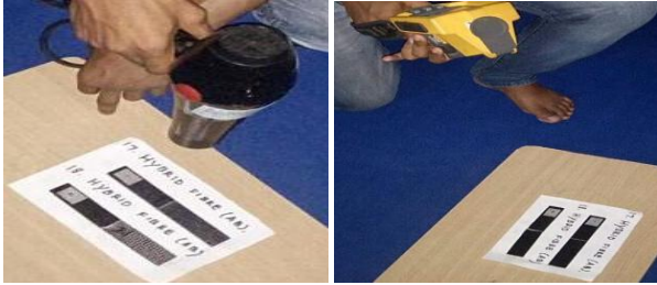
Fig. 9: Heating of specimen by hair drier (left) and thermographic image capture using IR camera (right)
