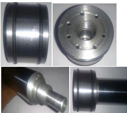
Fig. 4: Manufactured components and assembly of MR damper
