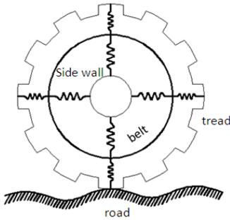
Fig. 1: Schematic diagram of tyre ride model
