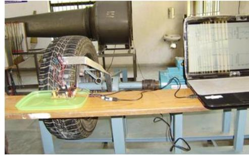
Fig. 3: Experimental test set up for measuring vibrations of rotating tyre
