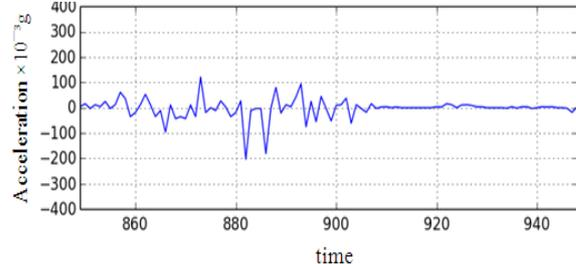
Fig. 6: X-axis (left) and Y-axis (right) acceleration for tyre rotation at 15Hz with 5kg load
