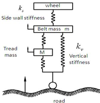
Fig. 2: Mathematical model of rolling tyre
