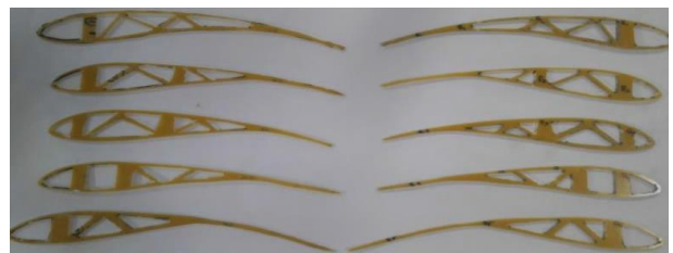
Fig. 6: Air foil sections cut through glass fibre
