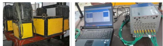
Fig. 14: Platform under load and data acquisition system
