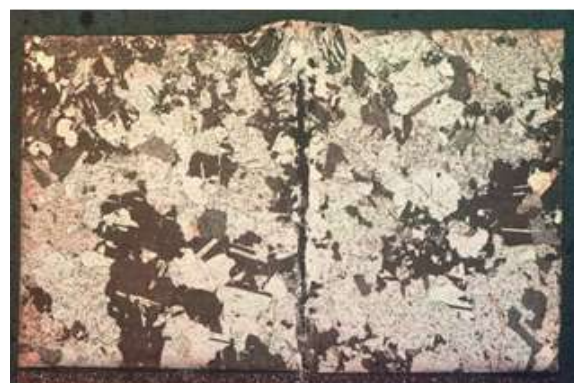
Fig. 4: Microstructure for EBW Cu-Cr-Zr samples
