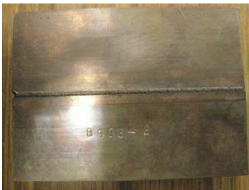
Fig. 3: EBW Cu-Cr-Zr-Cu-Cr-Zr plate samples
