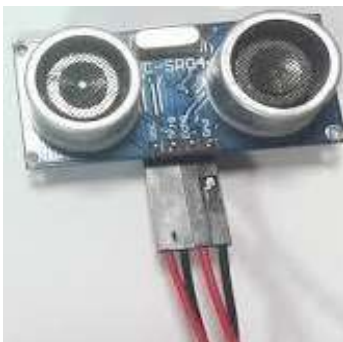
Fig.4: Close-up view of ultrasonic sensor used in the model
