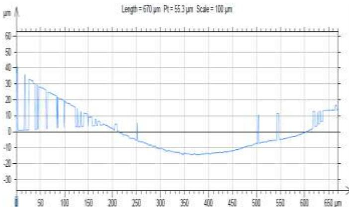
values are fixed: applied voltage is 8V, current is 2A, electrolyte concentration is 20g/lit and duty cycle is 40%. The given duty cycle value is low as opposed to the high values required. The current at its lowest point also plays a factor in reducing the overall quality of the surface. Duty cycle should be the major factor due to which poor surface finish is obtained in this material.
