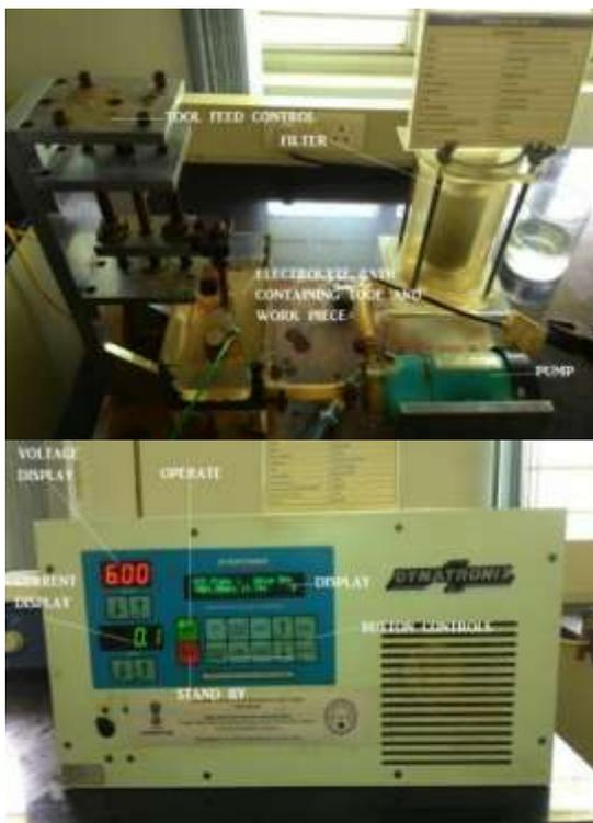
Fig. 1: Micro ECMM setup and pulse rectifier
