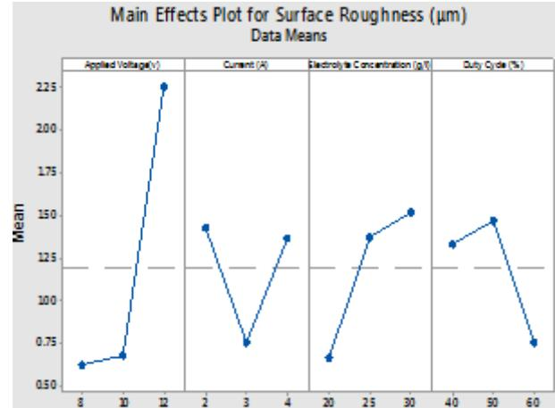
Fig. 4: Main effects plot for surface roughness
