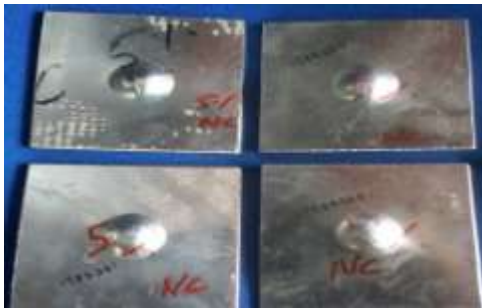
Fig.3: Specimens subjected to Erichsen cupping
