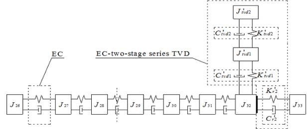
Fig. 11(b): Two-stage series TVD and EC
