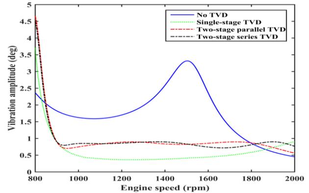
**Fig. 7: Vibration amplitudes at the input end of rear axle**
