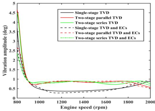
**Fig. 12: Vibration amplitudes at the input end of rear axle**
