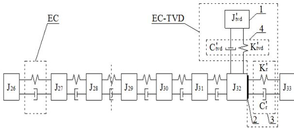
Fig. 9: Schematic diagram of installed position of EC and EC-TVD
