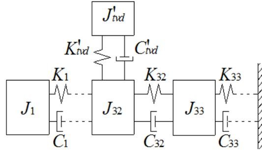
Fig. 5: Mechanical model of the matched MDOF system including single-stage TVD
