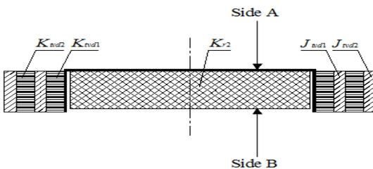
Fig. 10(b): Elastic coupling coupled to two-stage parallel TVD
