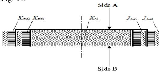
Fig. 10(a): Elastic coupling coupled to two-stage series TVD
