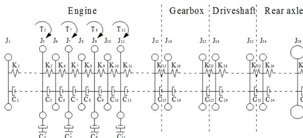
Fig. 2: VPTS torsional vibration model
