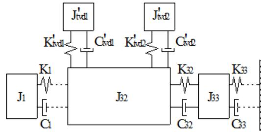
Fig. 6(a): Two-stage parallel TVD
