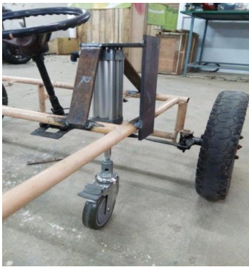
Fig. 5: Pneumatic cylinder with secondary roller
