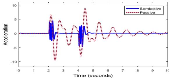
Fig. 10: Comparison of acceleration of head for passive and semi-active suspension model
