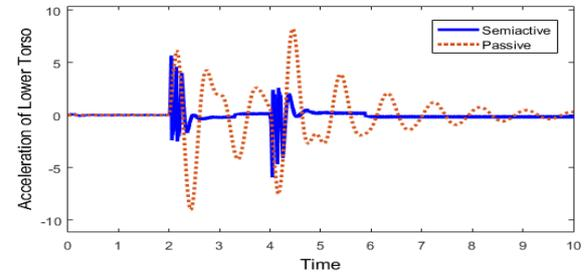
Fig. 12: Comparison of acceleration of lower torso for passive and semi-active suspension model
