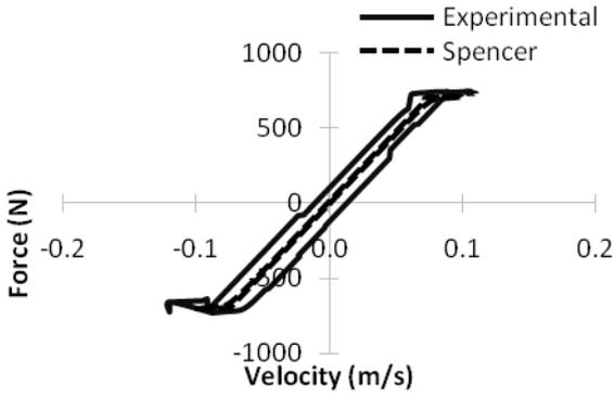
Fig. 6: Comparison of force vs. Velocity of Spencer model for MATLAB/SIMULINK and experimental analysis
