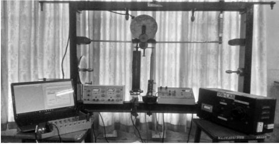
Fig. 1: Experimental setup for testing MR damper
