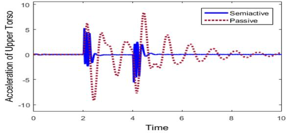
Fig. 11: Comparison of acceleration of upper torso for passive and semi-active suspension model
