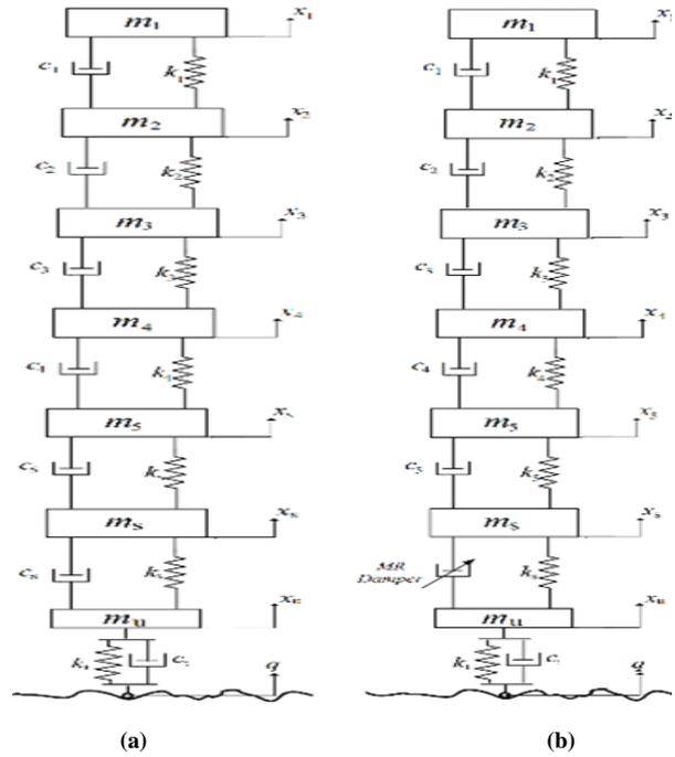
Fig. 7: Quarter car Suspension with human body lumped mass model (a) passive (b) semi-active with MR damper
