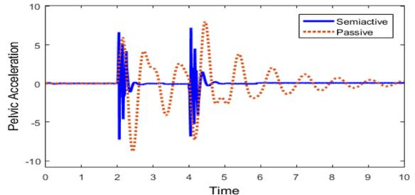
Fig. 13: Comparison of Acceleration of pelvis for passive and semi-active Suspension model
