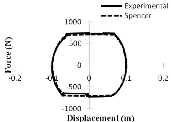
Fig. 5: Comparison of force vs. Displacement of Spencer model for MATLAB/SIMULINK and experimental analysis
