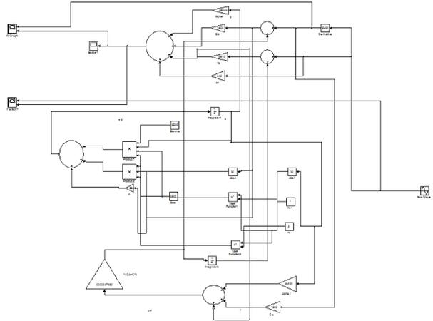
Fig. 3: Simulink modelling of phenomenological Spencer model of MR damper
