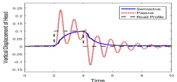
Fig. 14: Comparison of vertical displacement of head for passive and semi-active suspension model
