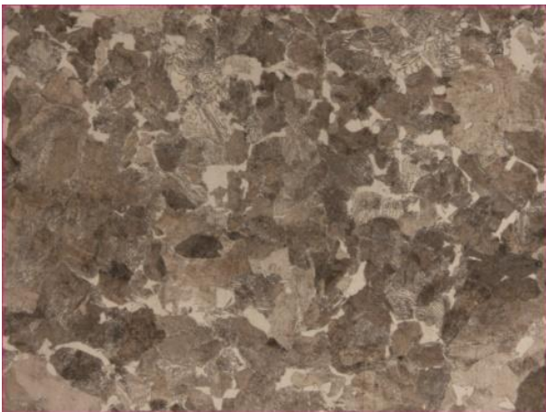
Fig. 3: Microstructure of normalized AISI 1050
