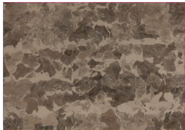
Fig. 2: Microstructure of annealed AISI 1050
