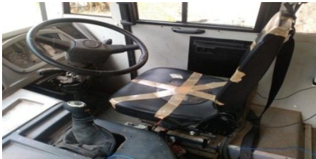
Fig. 1: Accelerometer location on driver seat
