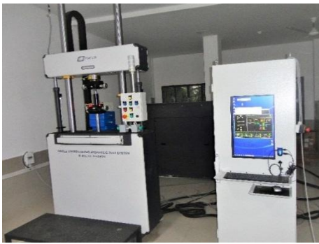
Fig. 1: Experimental setup for testing MR damper
