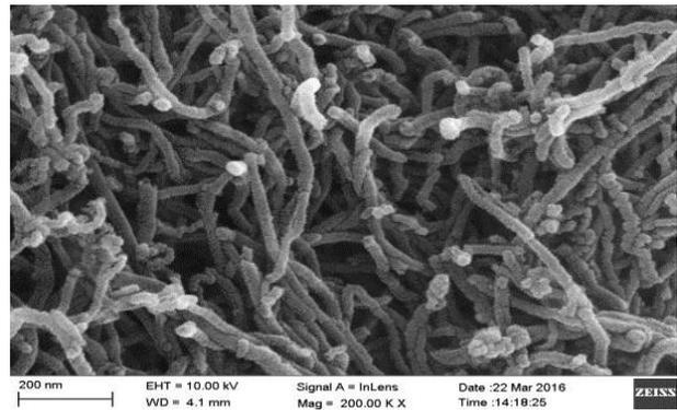
**Fig. 2: Micro-structure of MWCNT at magnification of 200 K X**
