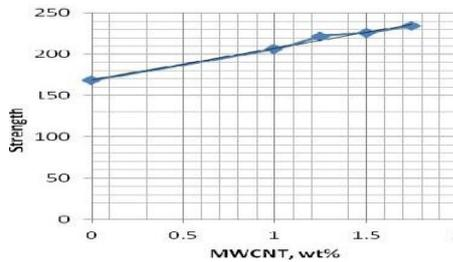
Fig. 8: Ultimate strength (MPa) vs. MWCNT wt%
