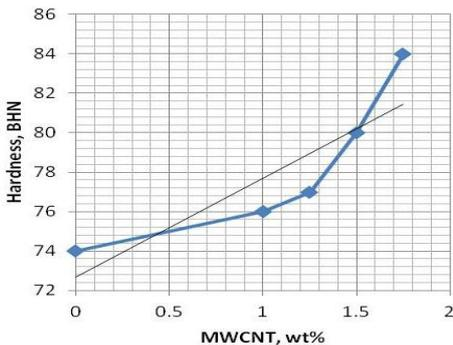
Fig. 6: Hardness vs. MWCNT
