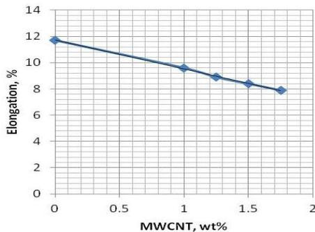
Fig. 10: Elongation vs. MWCNT wt%
