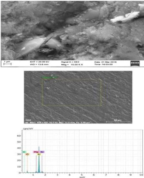
Fig. 5: ED-X of 1.75 wt% MWCNT with strong reflection peak
