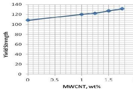
Fig. 9: Yield strength (MPa) vs. MWCNT wt%
