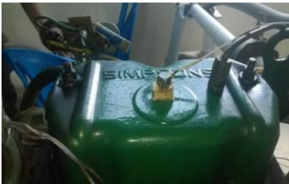
Fig. 4: Sensor mounting on engine head
