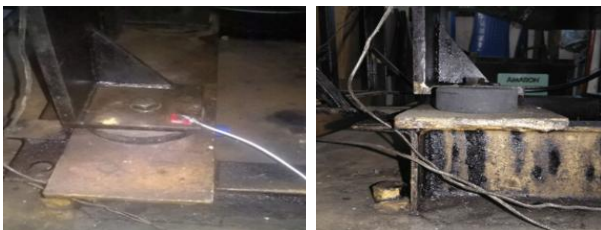
Fig. 5: Clamping of fluorocarbon and rubber mounts
