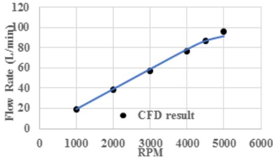
Fig. 7: Volumetric flow rate vs. RPM (configuration 1)
