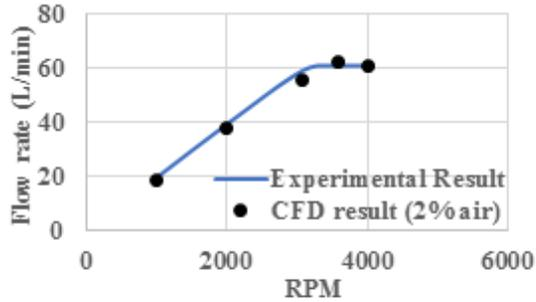
Fig. 8: Volumetric flow rate vs. RPM (configuration 2)
