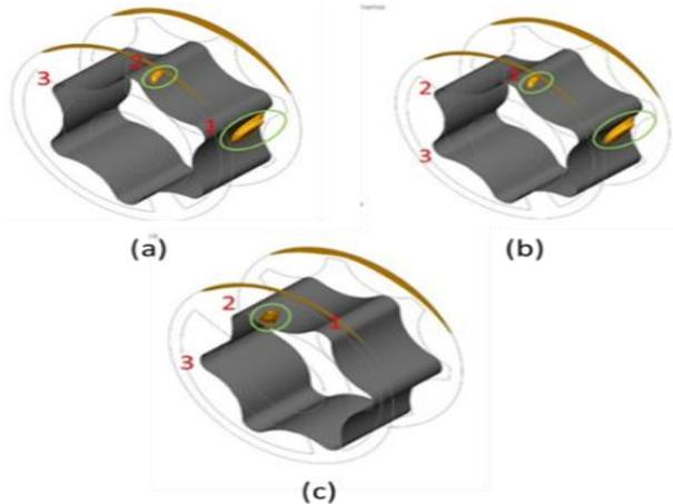
Fig. 11: Iso-fractions of 0.1 Vapour volume fractions
