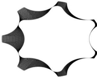
**Fig. 4: Rotor volume cross section**
