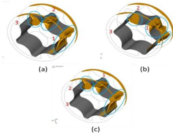
Fig. 12: Iso-fractions of 0.5 total gas volume fraction
