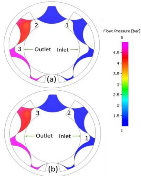
Fig. 9: Pressure contours
