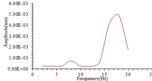
Fig. 13: Displacement of transport utility vehicle in Z-direction
