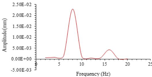
Fig. 11: Displacement of transport utility vehicle in X-direction
