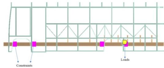
Fig. 4: Boundary conditions applied to meshed model
