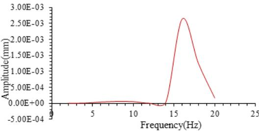
Fig. 12: Displacement of transport utility vehicle in Y-direction
