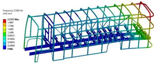
Fig. 5: First mode shape of transport utility vehicle
