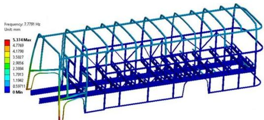
Fig. 7: Third mode shape of transport utility vehicle
