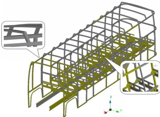
Fig. 3: Meshed model of the vehicle with modified dimensions
