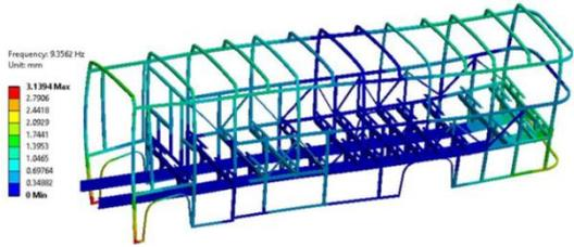
Fig. 10: Sixth mode shape of transport utility vehicle
