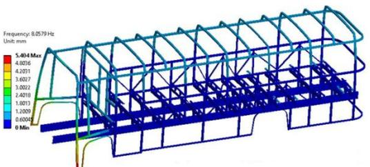
Fig. 8: Fourth mode shape of transport utility vehicle
