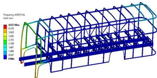
Fig. 6: Second mode shape of transport utility vehicle
