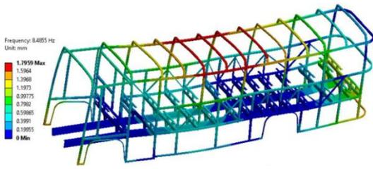
Fig. 9: Fifth mode shape of transport utility vehicle
