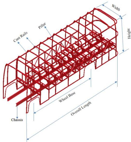
Fig. 2: Dimensional details of transport utility vehicle
