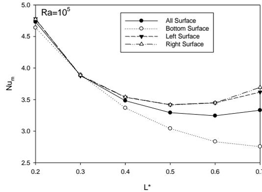
Fig. 4(b): Avg. Nu vs. Length ratio ( $K^*=1, \phi=0.04$ ) at  $Ra=10^5$
