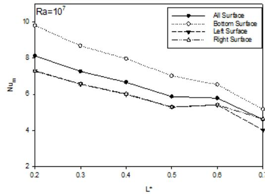
Fig. 4(c): Avg. Nu vs. Length ratio ( $K^*=1, \phi=0.04$ ) at  $Ra=10^7$
