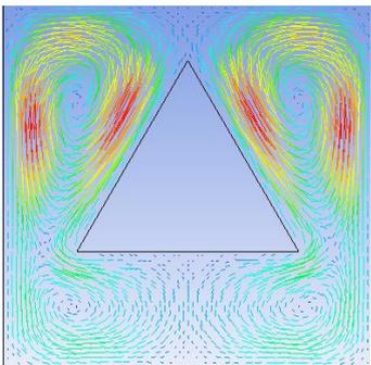
Fig. 3(c): Velocity vector ( $K^* = 1, \phi = 0.04$ ) at  $Ra=10^5$  and  $B=0.6$
