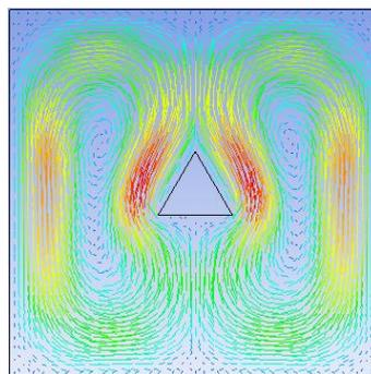
Fig. 2(a): Velocity vector (K\* = 1, φ = 0.04) at Ra=10<sup>3</sup> and B=0.2
