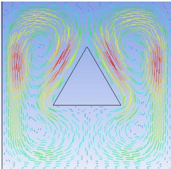
Fig. 3(b): Velocity vector ( $K^* = 1, \phi = 0.04$ ) at  $Ra=10^5$  and  $B=0.4$
