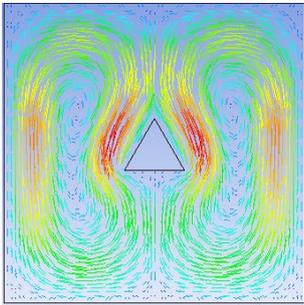
Fig. 3(a): Velocity vector ( $K^* = 1, \phi = 0.04$ ) at  $Ra=10^5$  and  $B=0.2$
