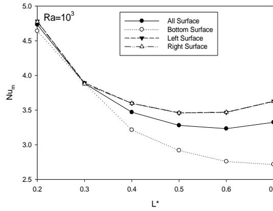
Fig. 4(a): Avg. Nu vs. Length ratio ( $K^*=1, \phi=0.04$ ) at  $Ra=10^3$
