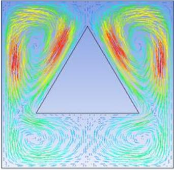
Fig. 2(c): Velocity vector ( $K^* = 1, \phi = 0.04$ ) at  $Ra=10^3$  and  $B=0.6$
