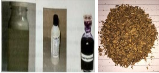
Fig. 1: (a) Unsaturated polyester resin (b) Catalyst MEKP (c) Accelerator cobalt naphthenate (d) Crushed walnut shell
