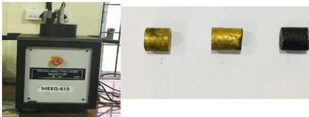
Fig. 5: Pin on disc apparatus and wear test specimens
