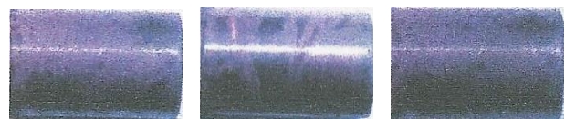
Fig. 4: Specimens after corrosion test - Left (1), Mid (2), Right (3)
