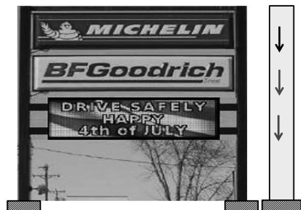
Fig. 9: Real life example of a frame with multiple sign boards (left), and the simplified axial loading of an 'equivalent bar' with multiple intermediate loads
