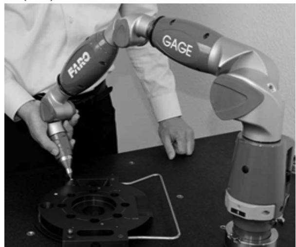
Fig. 5 : Vernier caliper and FARO GAUGE used for measurement of components
