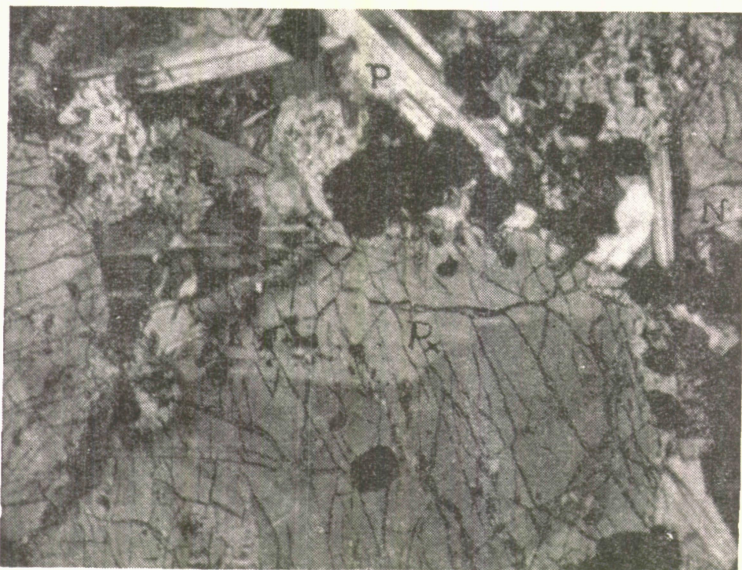
Figure 2a. Photomicrograph of theralite, showing zoned pyroxene (Px), plagioclase (P) and interstitial nepheline (N). Cross polars ( \times 25 ).
