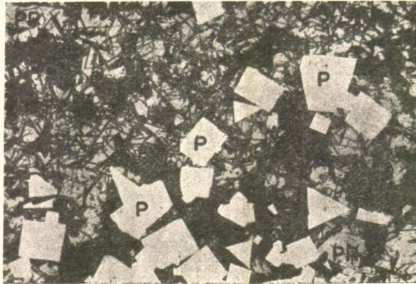
Figure 1. Idiomorphic pyrite (white) in pyrrhotite mass (grey). Black matrix is dolomite and chlorite.
