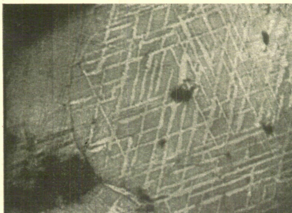
Figure 1. Exsolution intergrowth of linnaeite-millerite. Millerite (light grey) blades occupying three sets of cleavage planes in linnaeite (dark grey) \times 250 . Oil. Uncrossed.
