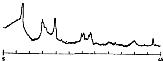
Figure A. Powder X-ray diffraction patterns of clay from Shivaganga.
