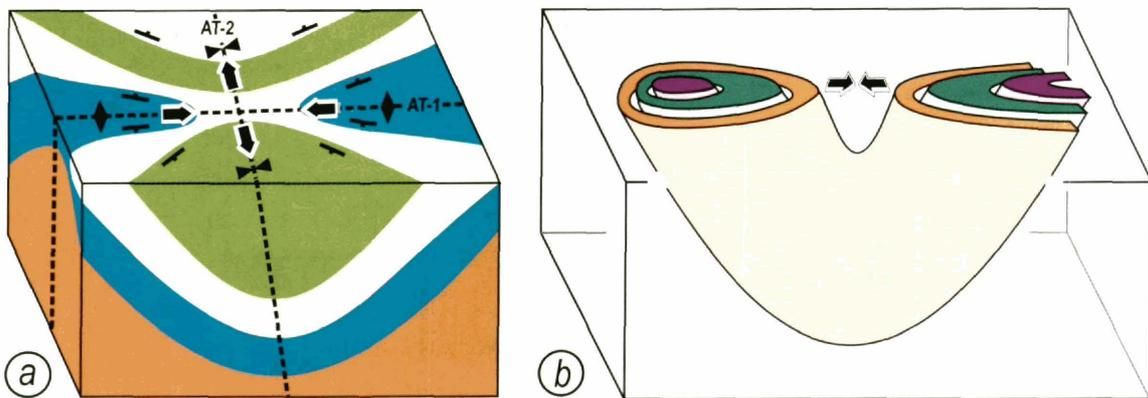
Fig.3. Three-dimensional geometry and outcrop pattern. (a) Type-1 interference structure (based on fig. 15.6 in Ghosh, 1993, p. 337). AT-1 and AT-2 are the axial traces of anticlinal and synclinal hourglass structures. Arrow-plunge direction. (b) Sheath fold. Arrows indicate reversal in plunge direction due to hinge line inversion.
