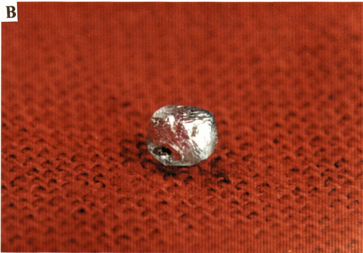
Fig.2. (A). Outcrop of Wairagarh conglomerate showing highly deformed clasts. (B). Octahedral gem quality diamond grain recovered from the conglomerate matrix (length 3.5 mm, breadth 2.5 mm).
