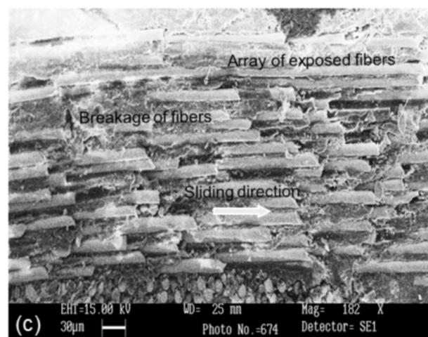
Fig. 5 SEM image of the worn specimen of rice husk filled glass-epoxy composites for a sliding distance of 3000 m at sliding velocity of 1 m/s and applied normal load of (a) 10 N; (b) 20 N and (3) 30 N
