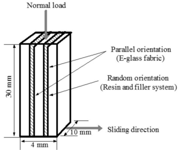
Fig. 2 Schematic illustration of fibre orientation and subjected loads on test spec
