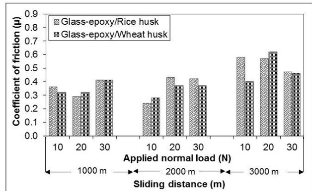
Fig. 4 Variation of coefficient of friction with applied normal loads for sliding distance of 1000, 2000 and 3000 m
