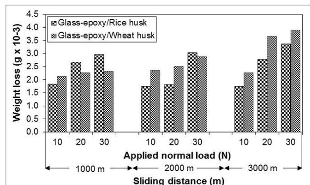
Fig. 3 Variation of weight loss with applied normal load for sliding distance of 1000, 2000 and 3000 m
