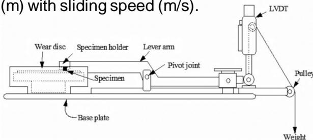
Fig. 1 Schematic diagram of the pin-on-disc tribo test machine
