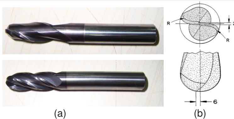
**Fig. 1** Ball nose end mill geometry (a) photograph and (b) end and side view of the tool
