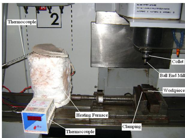
**Fig. 2** Experimental setup of ball end milling of preheated Inconel 600
