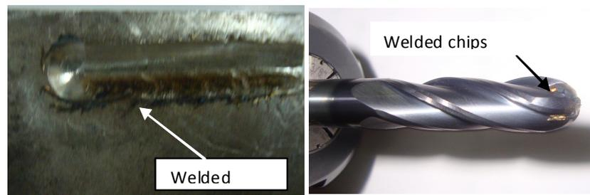
**Fig. 4** Surface image of the groove machined and a BUE attached to the ball end mill
