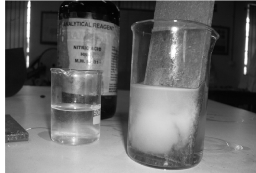
Fig.7: MS plate deburring by nitric acid solution [13]
