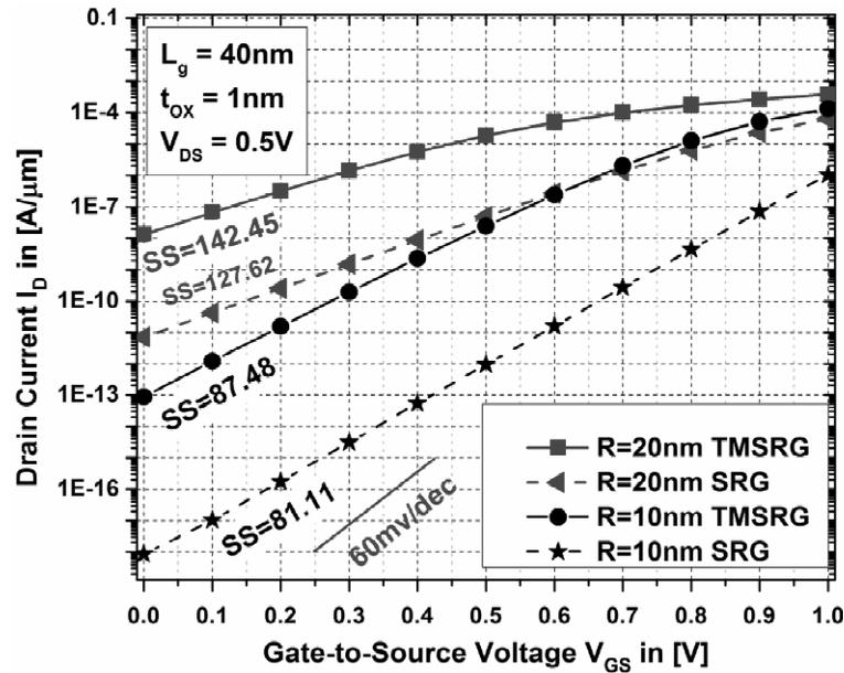
**Fig. 4:** The dependence of the drain current  $I_D$  on gate-to-source bias  $V_{GS}$  with subthreshold slope (SS) in mv/dec marked for different values of radius  $R$  ranging from 15nm to 50nm with  $V_{DS}=0.5V$ ,  $L_g=40nm$  and  $t_{ox}=1nm$
