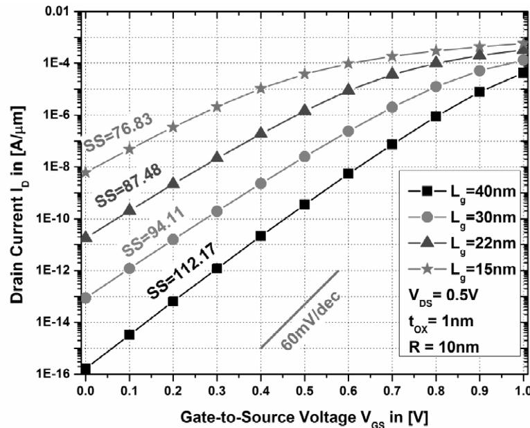
**Fig. 5:** The dependence of the drain current  $I_D$  on gate-to-source bias  $V_{GS}$  with their corresponding subthreshold slope (SS) in mv/dec marked for different values of gate length  $L_g$  ranging from 15nm to 40nm with  $V_{DS}=0.5V$ ,  $R=10nm$  and  $t_{ox}=1nm$
