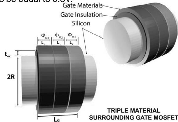
**Fig. 1:** 3-D device structure of TMSRG MOSFET
