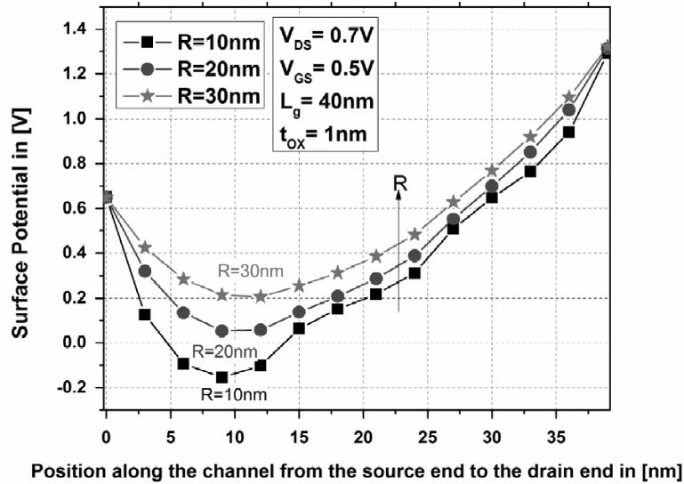
**Fig. 2:** Variation of Surface Potential as a function of position along the surface of the channel from the source end to the drain end for variable values of radius  $R$  ranging from 10nm to 30nm with gate length  $L_g=40\text{nm}$ , oxide thickness  $t_{ox}=1\text{nm}$ ,  $V_{GS}=0.5\text{V}$  and  $V_{DS}=0.7\text{V}$
