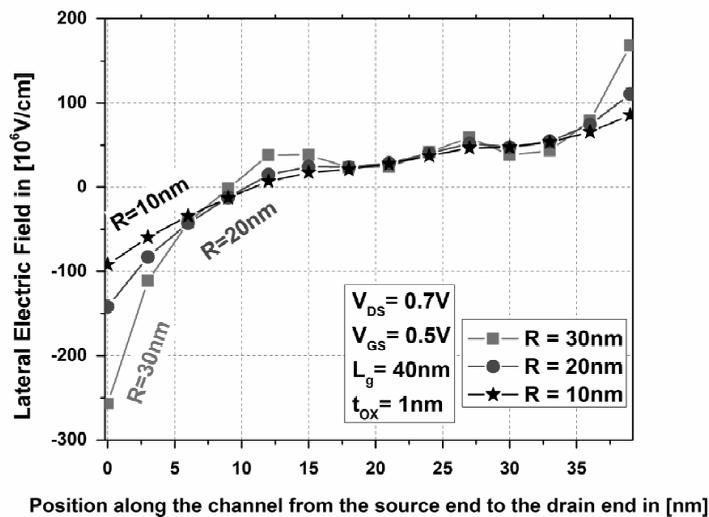
**Fig. 3:** Variation of lateral Electric Field as a function of position along the surface of the channel from the source end to the drain end for a TMSRG device with gate length  $L_g=40\text{nm}$ , oxide thickness  $t_{ox}=1\text{nm}$ ,  $V_{GS}=0.5\text{V}$ ,  $V_{DS}=0.7\text{V}$  for variable values of radius  $R$  ranging from 10nm to 30nm
