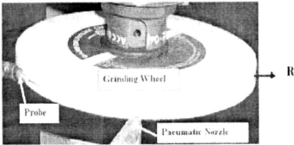
Fig. 1. The pneumatic barrier set up
