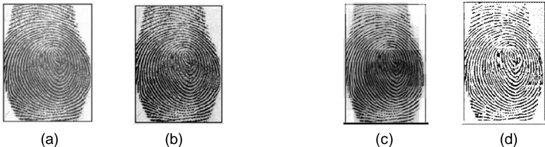
Fig 5: (a) Reference image for matching; (b) Output after performing Histogram equalization on reference image; (c) Enhanced image after doing FFT on image shown in Fig. 5(b); (d) Output after doing binarization on enhanced image i.e., Fig.5(c)
