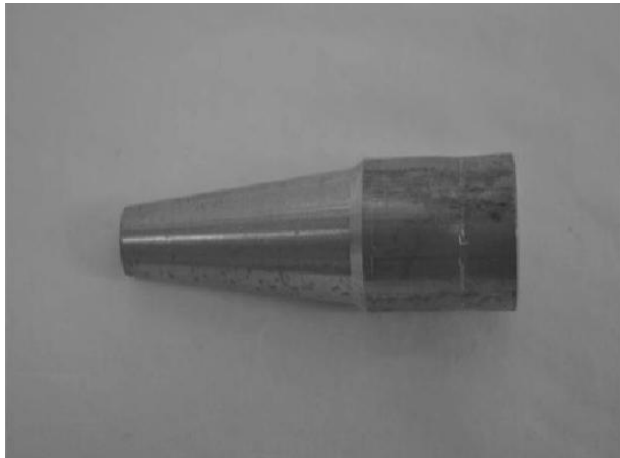
Fig. 3: Flood type copper cooling nozzle
