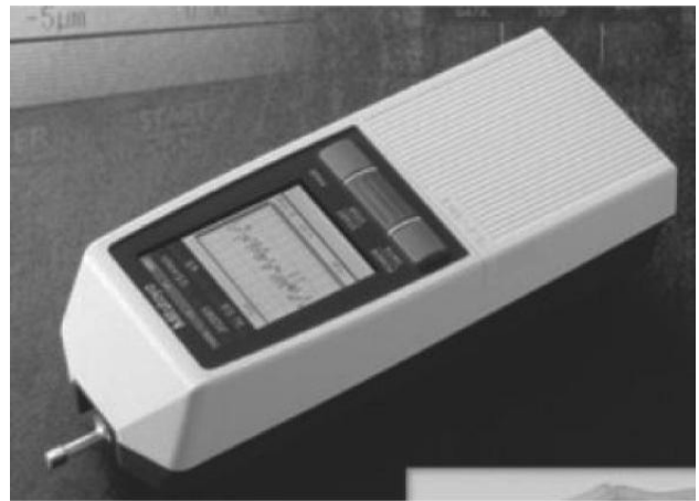
Fig. 4: Mitutoyo Surface Roughness Tester (Talysurf)
