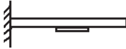
Fig 1: Cantilever beam with embedded Piezo patch at the middle
