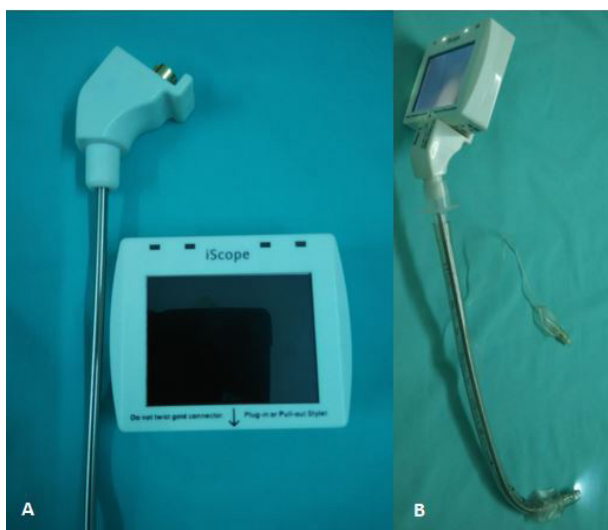
Figure 1. I-scope A. I-scope monitor and Stylet, B. Endotracheal Tube mounted on I-Scope.
