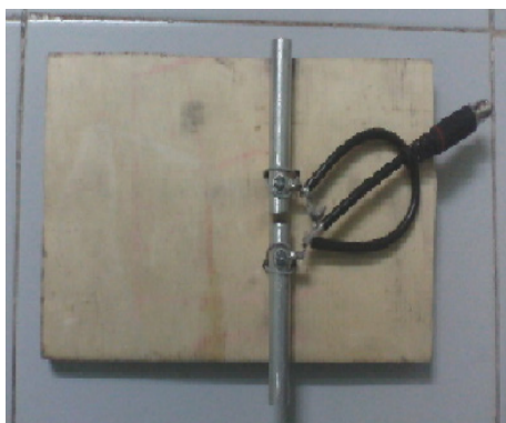
Fig 1: Dipole with length 16cm tuned at 879MHz
