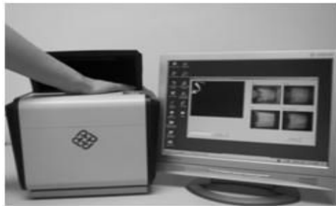
Figure 3: An outlook of multispectral palm print image acquisition device
