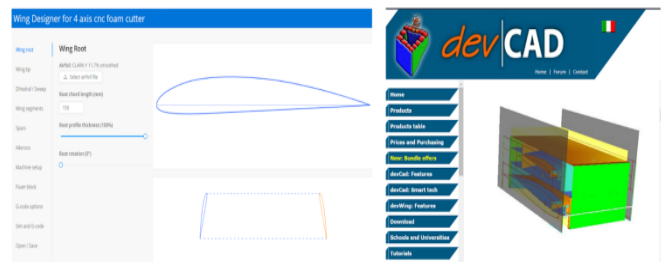
These are software generates G Code as per the given aerofoil shape for the CNC foam Cutter
