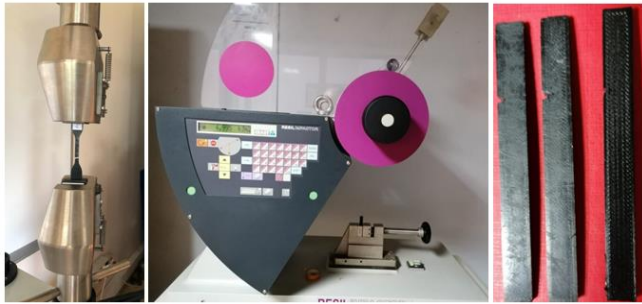
Figure 3. Tensile tests and Izod impact test devices
