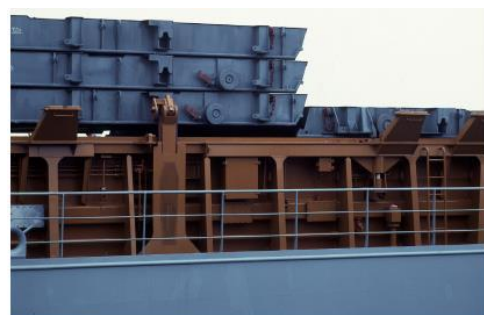
Figure 3. Stacking Hatch Covers [1-10].
