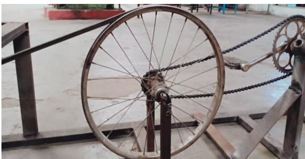
Figure 1: Mechanism for transfer of torque from pedal to tub
