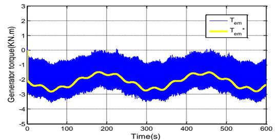
Figure 5. DFIG Torque and its reference.
