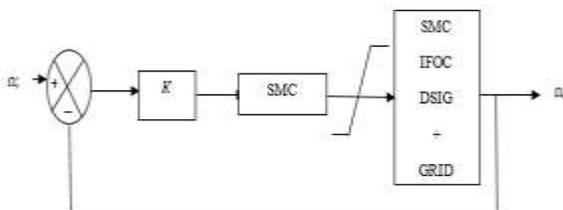
Figure 2. Basic structure of the sliding mode controller for indirect field oriented control of DSIG.
