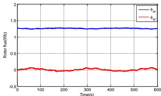
Figure 6. Direct and quadratic rotor flux.
