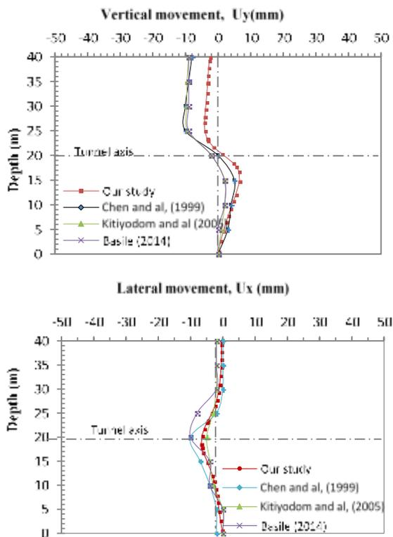
**Figure 2.** Computed soil vertical and lateral movements at  $x=4,5m$
