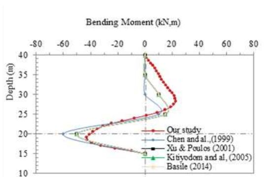
**Figure 4.** Single Pile Bending moment and Axial force
