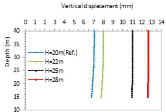
Figure 7. Computed single pile vertical responses for different tunnel depth H
