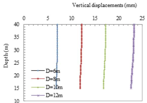
Figure 8. Computed single pile vertical responses for different tunnel depth H
