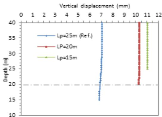
Figure 6. Computed single pile vertical responses for different length pile  $L_p$
