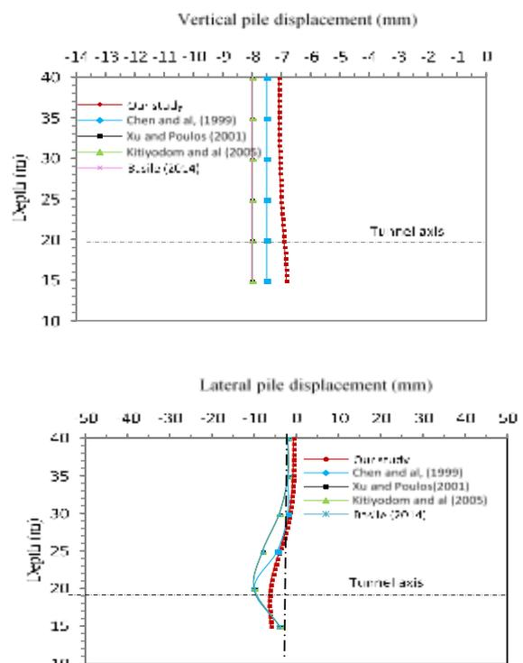
**Figure 3.** Computed vertical and lateral single pile response at  $x=4,5m$
