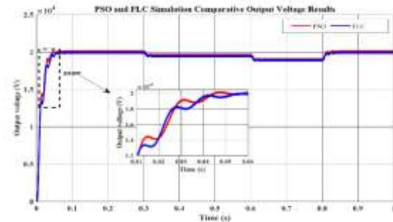
Figure 18. The Boost output Voltage Results of PSO algorithm and FLC.
