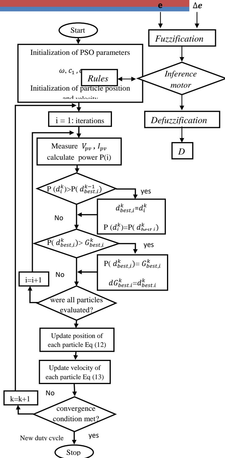
Figure 4. Flowchart of modified the MPPT PSO algorithm.
