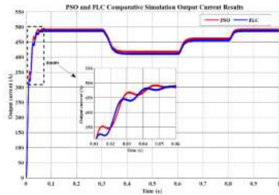
Figure 12. The Boost output Current Results of PSO algorithm and FLC.
