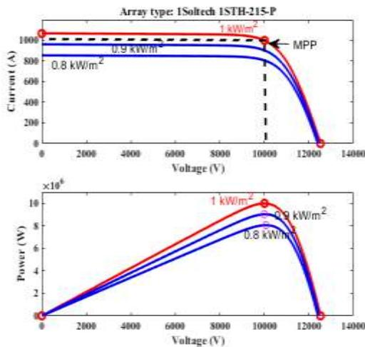
Figure 2. I-V and P-V characteristics of PV array.
