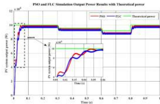
Figure 19. The Boost output Power Results of PSO algorithm and FLC.
