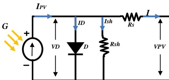
Figure.1. Equivalent circuit for a PV cell.
