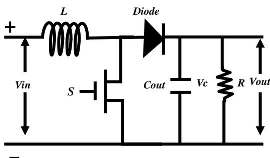
Figure 3. DC-DC Boost Converter.
