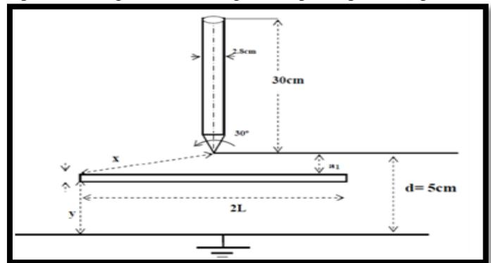
Fig .1.Point-barrier system
