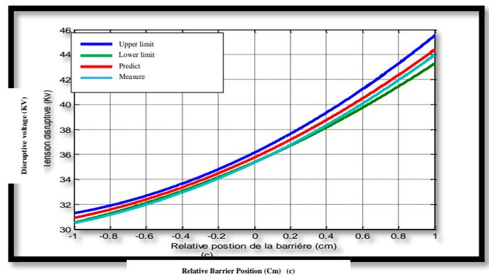
Fig.3. Influence of the relative position of the barrier on the breakdown voltage different width (a) of 5 cm, (b) 10 cm and (c) of 15 cm, in alternating voltage (50 Hz)
