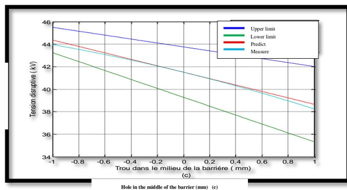
Fig. 4. Influence of barrier width on breakdown voltage: Different position in alternating voltage (50 Hz)
